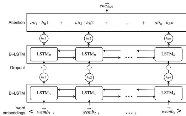
Fig. 3. Our network architecture to produce document encodings. The word embeddings pertaining to the input text are passed through two bidirectional LSTM layers. Finally, an attention layer is used to obtain the final document encoding. This layer is an implementation of the attention mechanism described in [13].
