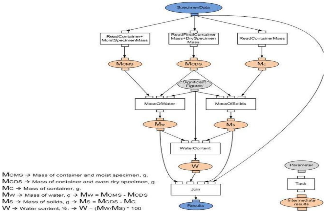
Fig. 4. ASTM D2216-5122 Protocol as Workflow
